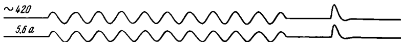
Fig. 19. Oscillograms of current strength and voltage during control measurement on a standard resistance of 420 \Omega alternating current and of a discharge current (capacity 24 \mu\text{f} , inductance 0.25 H) when the potential difference at the condenser is 3000 v.
