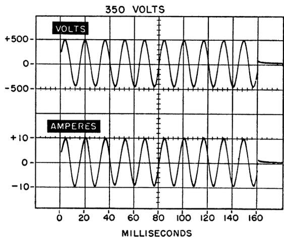
TEXT-FIGS. 1A and B. Discharge waveforms of the two defibrillators employed in the present study, A) DC or capacitor discharge at a setting of 70 WS, and B) AC at setting of 350 V. Both of these settings represent levels effective for transthoracic defibrillation of the dog heart.
